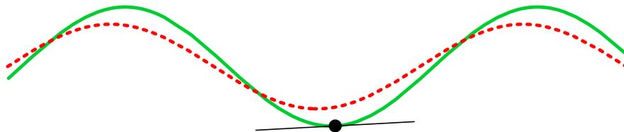
Now we know that the red track is the rear wheel. Which way was the bicycle moving? Here is a picture with some tangents drawn to the red track.
