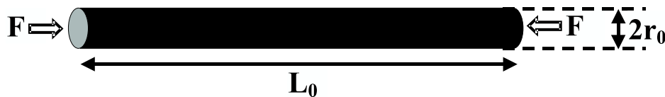
Fig. 3.1: A bar under compression.
