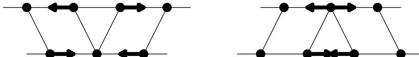
Figure 7. The scattering rules for our dynamical geometry LGA: An edge is created when two particles advect to the same lattice point and an edge is deleted if after advection each endpoint is occupied by a single particle with outward momentum.
