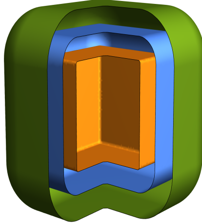
Figure 4: Examples of exaggerated \epsilon -rounding in blue and green of the cuboid interface in orange.
