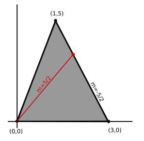
The red line is the line from the threat point (0,0) with slope equal to the negative of the slope along the Pareto optimal curve. The solution is the intersection of the red line and the line segment between (1,5) and (3,0). The first line has equation  $y = \frac{5}{2}x$  and the second line has equation  $y = -\frac{5}{2}(x-3)$ . The intersection is at x = 3/2, y = 15/4.
